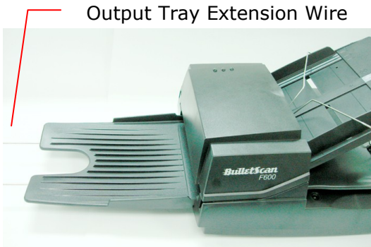
Figure 2-4 Install the ADF Output Paper Tray
